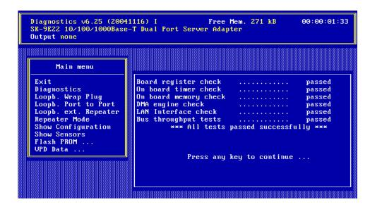
Figure 7. Typical display after a successful test (loopback wrap plug)
